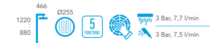
Myra Plus Telescopic Shower Column 2 Way Diverter-shower head and hand shower ● Chrome Chrome Hose (1,5 m.) 102158041EX Bath/Shower mixer should be bought separately.
