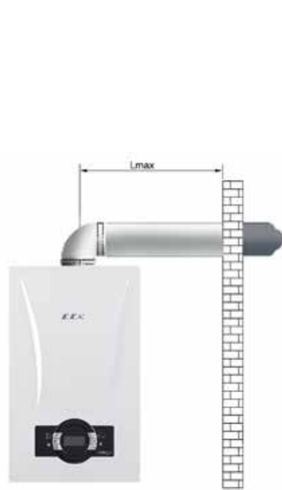
Horizontal Hermetic Flue Application L max. distance with single elbow: 10 m, Ø60/100 L max. distance with single elbow: 20 m, Ø80/125
