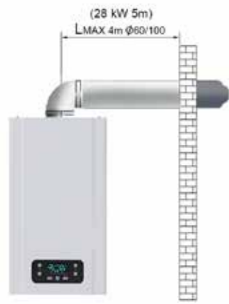
Horizontal Hermetic Flue Application
